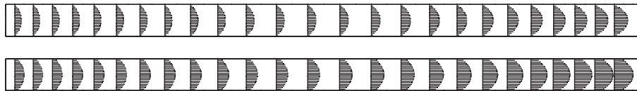
Figure 2. Velocity distribution along the straight micro channel with no-slip (upper) and slip-velocity (lower) boundary conditions.
